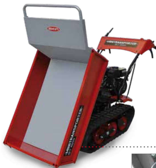
UNLOAD ANGLE up to 65 ° for a perfect emptying.
